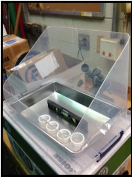
Figure 1 Solar still during construction.
